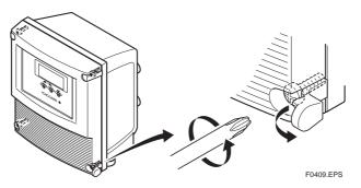
Figure 4.4.1 Removing the Front Cover
